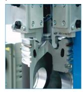
Automated inspection of camshafts.
