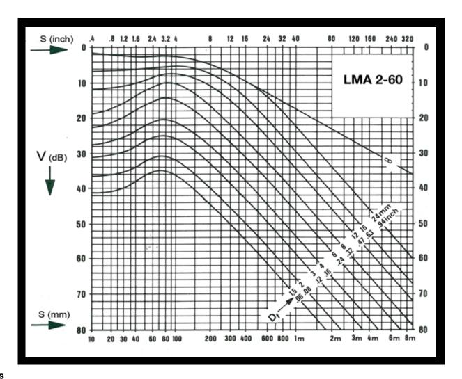
This Datasheet provides standard information about the supplied probe type. All numbers represent, or are based on, design standards - supplied probes will match these within an acceptable tolerance. Probes will normally be supplied with a calibration document detailing key parameters as measured for the actual probe.
