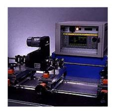
The ELOTEST PL.E is a compact universal instrument for fast test procedures during the manufacture of semi-fi nished products. It offers the same performance as the ELOTEST PL.1, but is limited to two channels and works autonomously or inconjunction with a host computer, PC or SPC.
