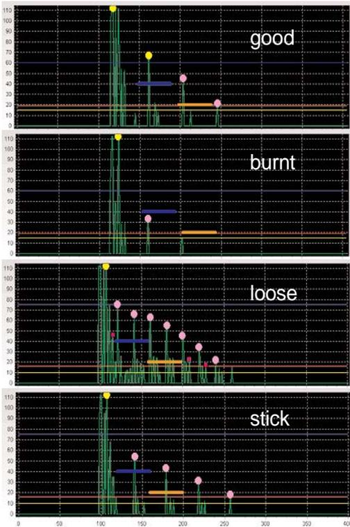
CYCLOPS performs CONVENTIONAL ultrasonic spot weld inspection, in automatic mode and with dry contact probes.
