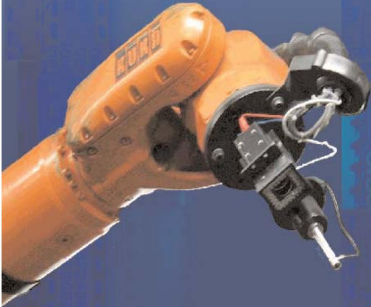
**CYCLOPS is a completely automatic in-line system for the inspection, evaluation and monitoring of spot welds via ultrasound and using artificial vision for position control**
