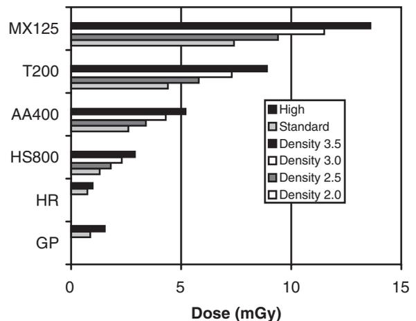
\* Flex GP and Flex HR Imaging Plates: dose required to reach highest ASTM and CEN System Classes at standard and high dose settings on ACR-2000/2000i readers.
