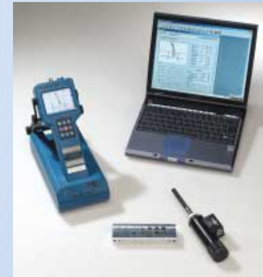
The docking station converts the one-hand instrument into a table-top instrument with a connector for PC or printer. By simply plugging it in, the intelligent charger electronics is activated and keeps the battery pack that is integrated in the instrument at its optimum load level.
