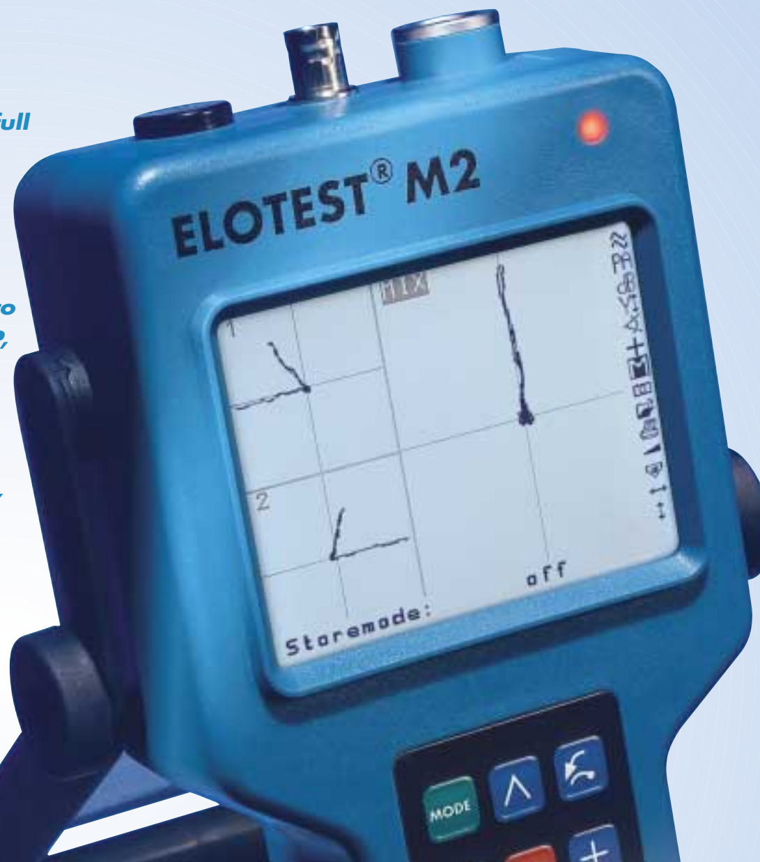
The ELOTEST M2 V3 allows all types of manual inspection beginning with the high-frequency crack detection of high-alloy components to medium-frequency crack and corrosion tests to low-frequency tests of multi-layer structures for stress cracks.
